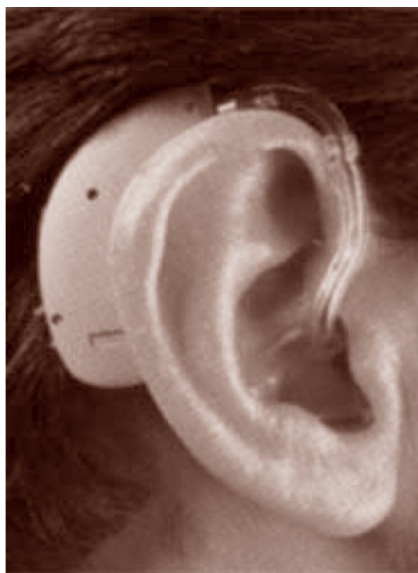
Figura 2. Auxiliares detrás de la oreja (BTE, Behind The Ear )
